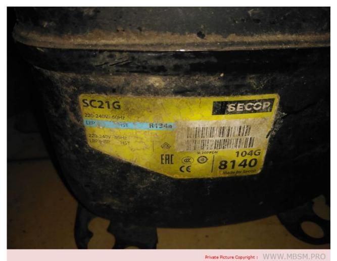
Mbsm.pro, Compressor, Secop, Original, New, 5/8HP, 470W, R134A, Refrigerator, Sc2lg, 104G8140
