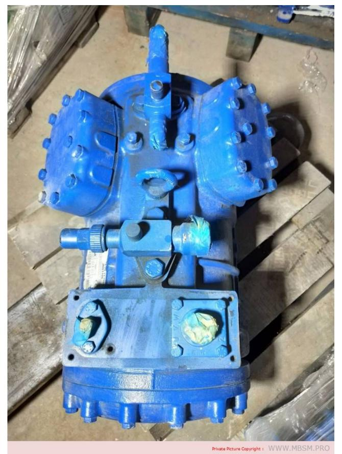
Mbsm.pro, Compressor, semi-hermetic, piston, Q4-24.1Y, Q4-24.1y1000, 4 hp, lbp
