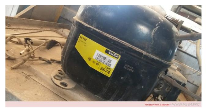
Mbsm.pro, Compressor, SC12C, 104L2674, DANFOSS,104L 2674, SC12C 104L2674, R22/R502, 3/8HP, 315W, MLbp, 1ph/220-240V/50HZ
