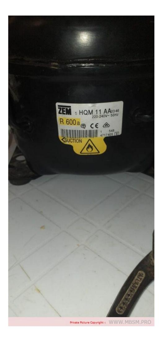
Mbsm.pro, Electrolux, Hermetic, Compressor, r600, LBP, CubiGel, Zem
