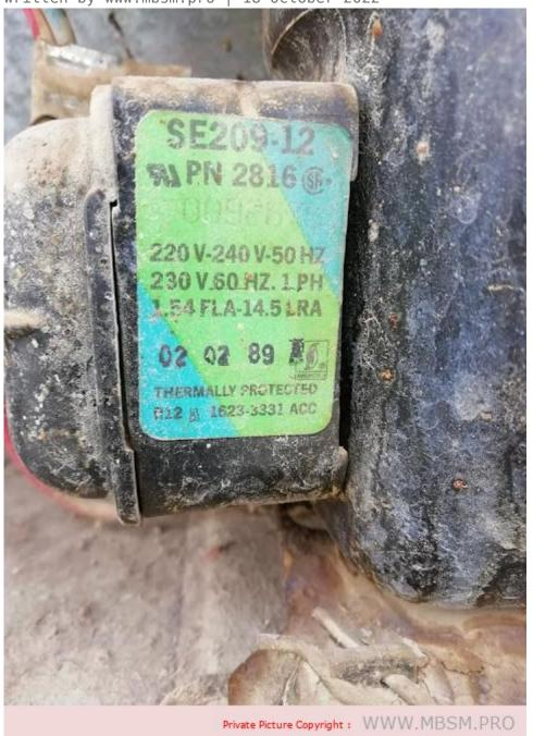
Mbsm.pro, American, Gibson, refrigerator, SE209-12, SE 209-12, SE209, R12, 527 L, 260 w, Compressor, 1/4 hp++, 1/3 hp-, AEA3430AXA / AEA4430AXA
