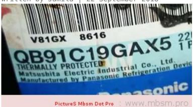
Mbsm.pro , Qb91c19gax5 ,Panasonic ,Compressor cooling , 1/4HP ,236W ,1Ph ,220V
