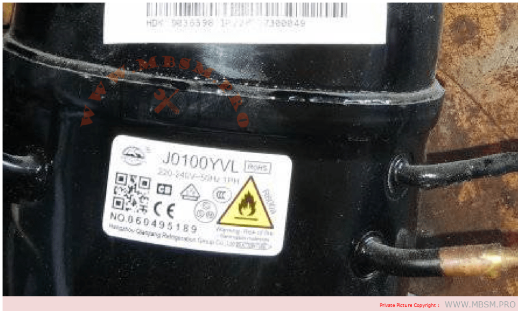
Mbsm.pro, Compressor, J0100YVL, jiaxipera, 100 w, LBP, R600a, 3 uf, e-ptc, 1/8 hp
