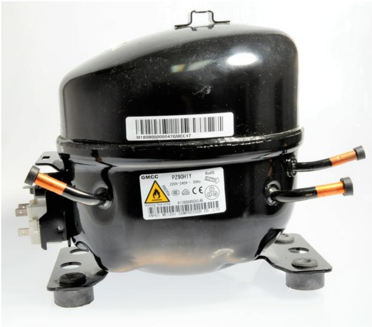
Mbsm.pro, Compressor, R600a, GMCC, Refrigerant, PZ90H1Y, SXF-562JA, 1/5hp, 167 W
