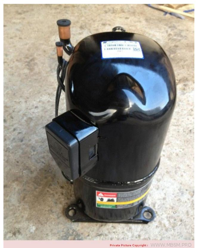
Mbsm.pro, Compressor, SFA5594EXG, SF100UT-006-A4, Taikang, 8 HP, 94000 btu/h, 460 v/60/3ph, 380 v/50/3ph, Replaces, ZR94KCE-TFD-250, ZR94KC-TFD-250, ZR94KC-TFD-950, Daikin , McQuay, 106647511 , 106647501, 50049004676, 0001222748, 30000110, Trane COM11182
