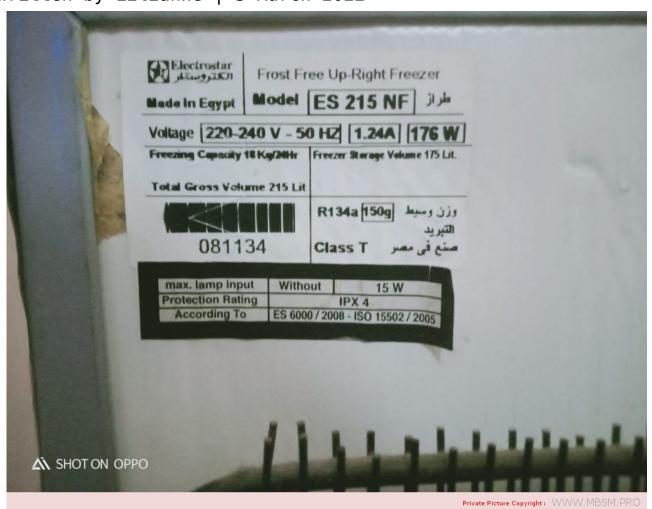
Mbsm.pro, Freezer, es215nf, Electrostar, five drawers, ES 215 P NF, Prestige, 215 L, Compressor, 1/5 Hp, r134a, 130 G, qbh66c13gpx, Panasonic
