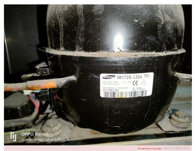
Mbsm.pro, Refrigerator, Fridge-Freezer, RT511JSPN, No Frost, Sumsung, 441 L, 309 L, Compressor, Mk172Q-L2U, 1/4 Hp, 205 W, 699 BTu/H, Samsung Compressor, Mk Serie, R134A, 7.21 cc, 220-240 v, LBP, Static Compressor, RSIR
