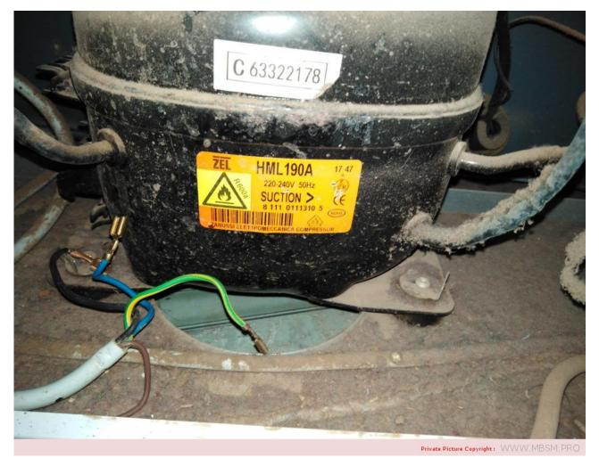
Mbsm.pro, Compressor, HML190a, 1/4 hp, zel, LBP, RSCR, Freezing compressor, R600a, 190 w, 163 kcal/h, run capacitor 3  $\mu$ F, aluminum wire
