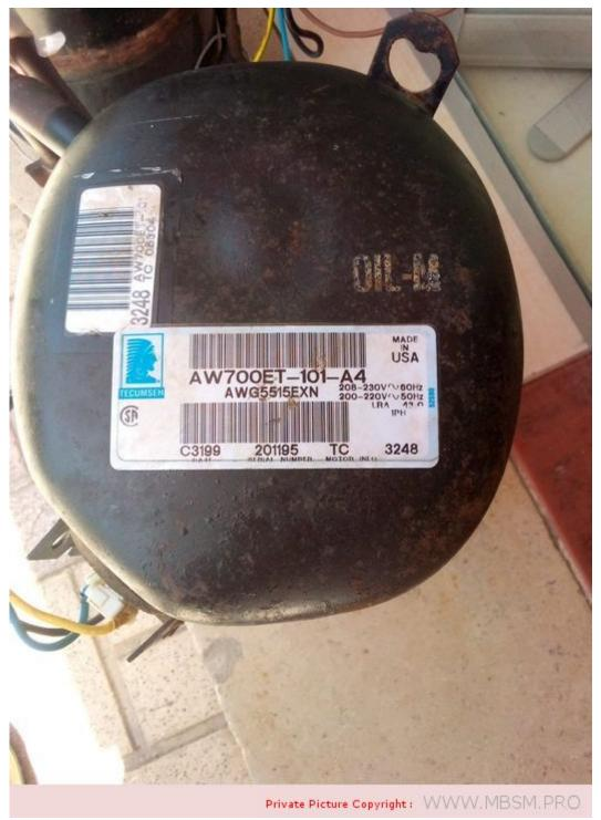
Mbsm.pro, Compressor, AW700ET-111-P2, Tecumseh 1-1/4 HP, 208-230V, 1 PH, 15,200 BTU, R22, Hermetic Compressor Replacement
