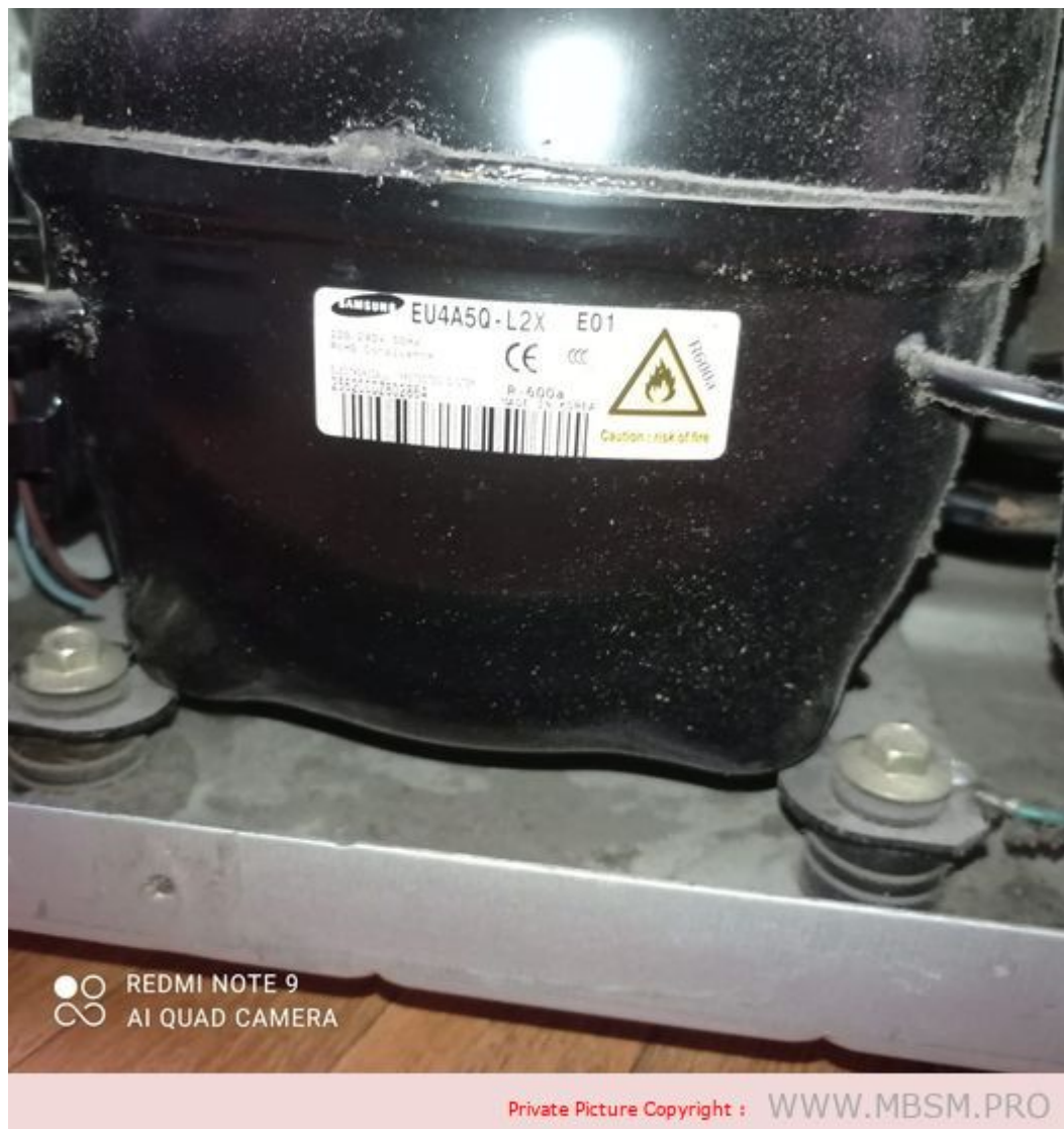
mbsm.pro, Samsung, Compressor, EU4A5Q-L2X, EU4A5QL2X, (VEGZ11C Compatible Embraco) , 1/4 hp, inverter, r600
