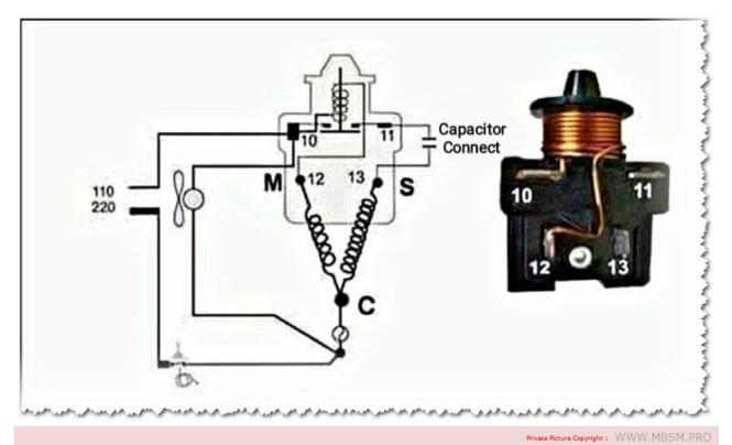
Mbsm.pro, Danfoss, compressor, relay, connection, Refrigeration
