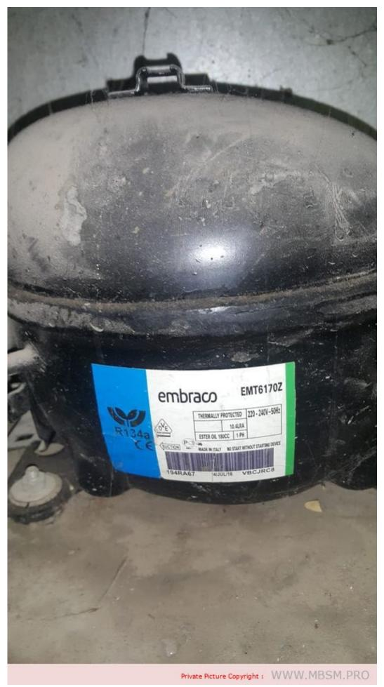
Mbsm.pro, Compressor, EMBRACO, EMT6170Z, HBP, R134a, 350 G, 220-240V/1F/50Hz,
