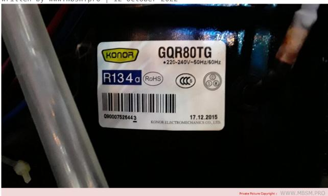
Mbsm.pro, Compressor, SIKELAN, GQR80TG, 1/4 hp++, HBP, 1/3 hp-, Refrigeration, R134a, 220-240V 50HZ, MQ-GQR80TG, GQR80TG
