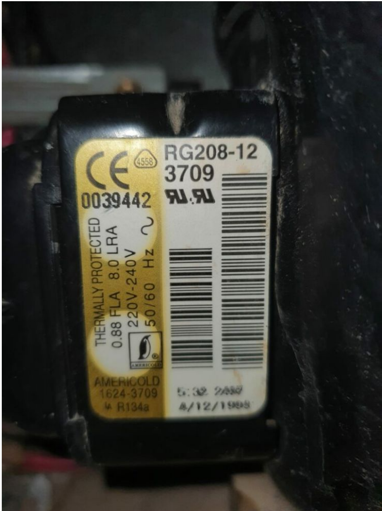
Mbsm.pro, Compressor, Rg208-12, R134a, 1/4 hp-
