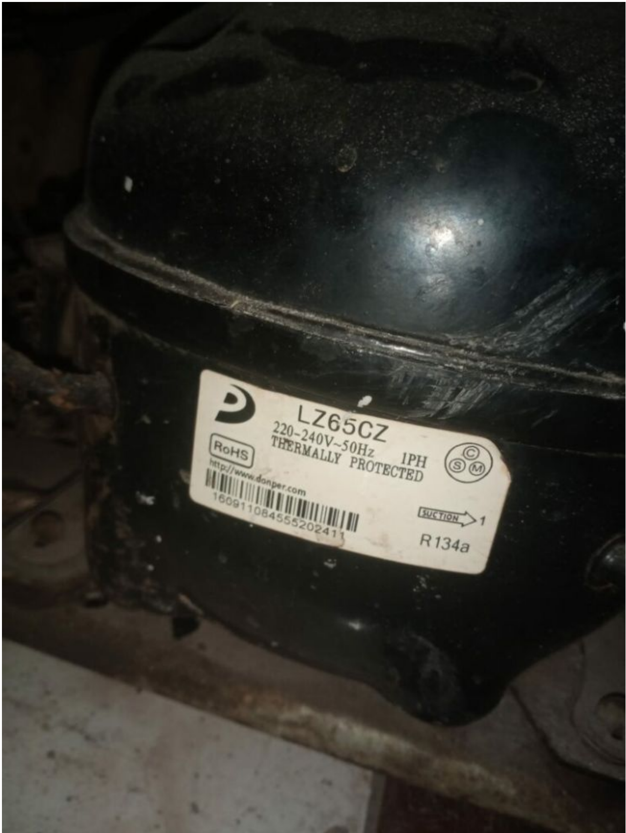
Mbsm.pro, Compressor, Lz65CZ, 1/5 hp, r134a
