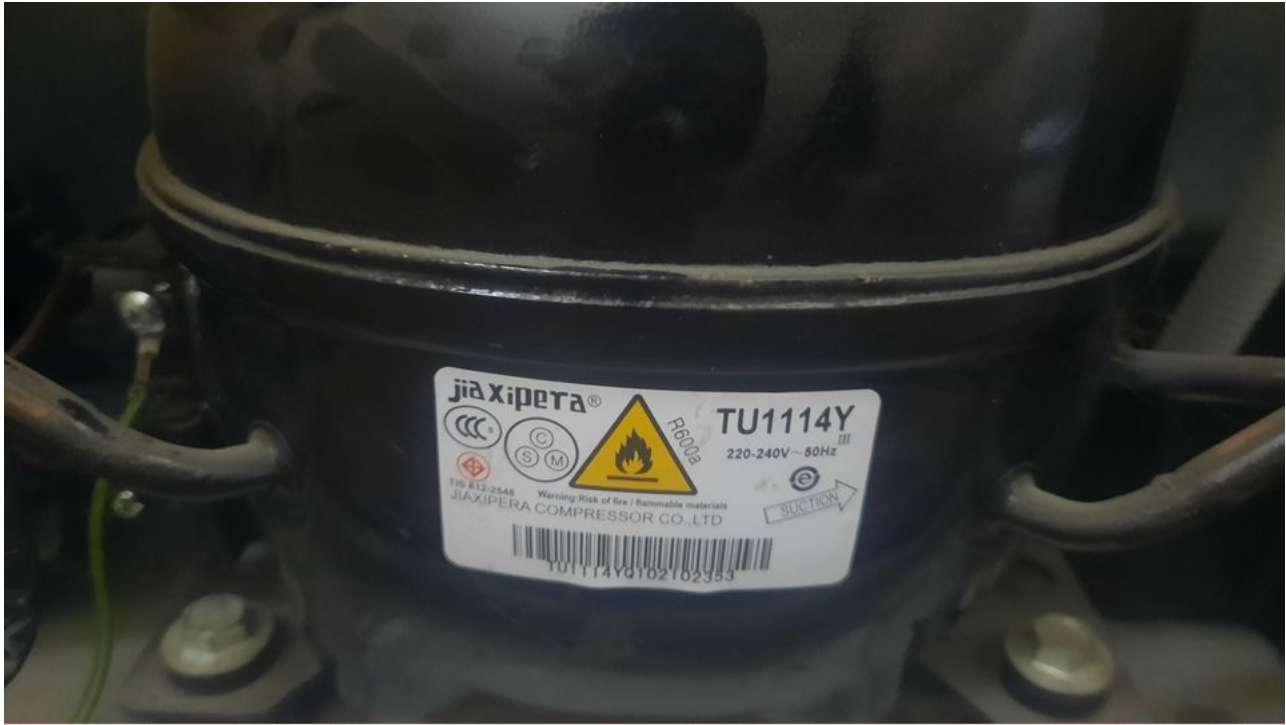
Mbsm.pro, Beko, Refrigerator, Compressor, TU1114Y, 1/4HP, R600A
