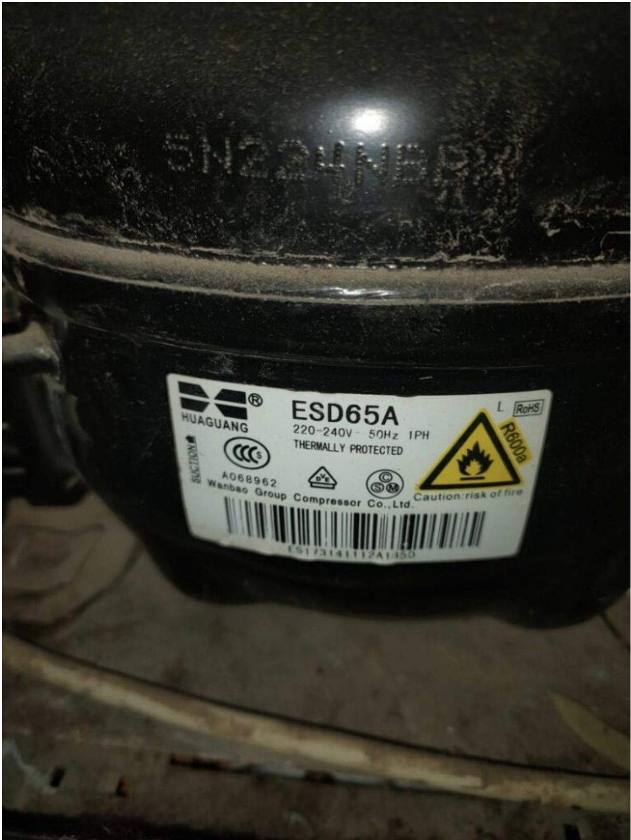
Mbsm.pro, Compressor, esd65a, 100 w, 1/8 hp, r600a
