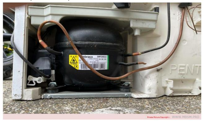
Mbsm.pro, Compressor, TLX4KK, 102h 4446, Compressor Mini Portable, R600A, Truck Car Fridge, 20-to-40 L, Compatible , EMY20CLC, 1/12 hp, Lbp, 54 W at  $23^{\circ}$ C, Capacitor  $2.5\mu$ F
