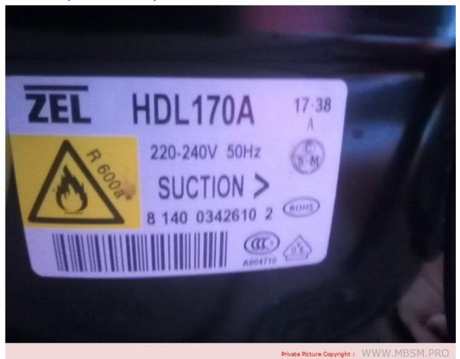
Mbsm.pro, Compressor, hdl170a, 1/5 hp, 172 w, aluminum winding, Capacitor 4  $\mu F,\ R600a$
