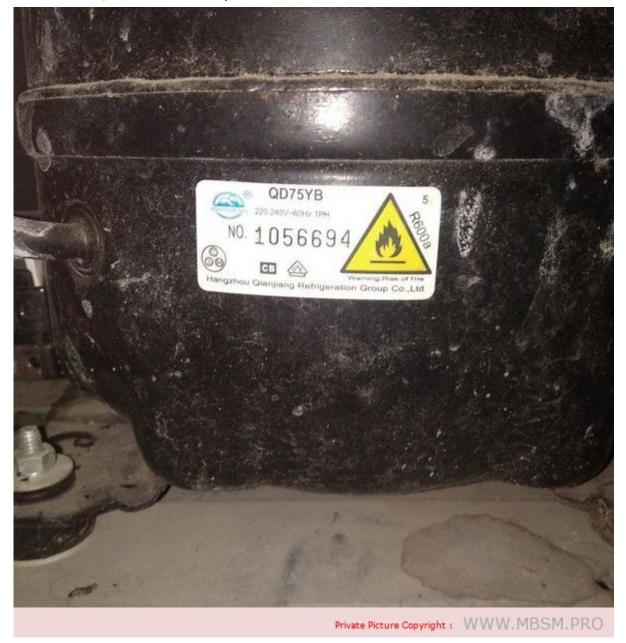
Mbsm.pro, Refrigerator, Electrolux, 308 Liters, Silver, Ert45g2hqi, Compressor, QD Compressor, R600a, QD75Y, 1/6HP, LBP
