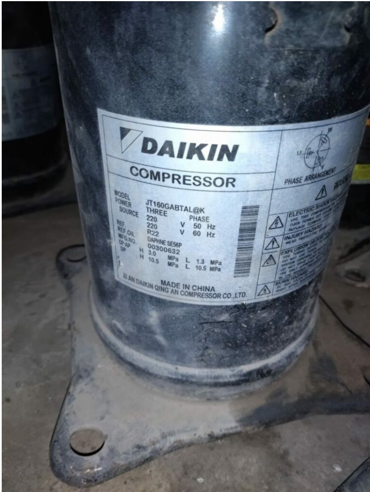
Mbsm.pro, compressor, jt160gabtal, 5 hp, 400 v, 3 ph, DAIKIN scroll, air conditioning
