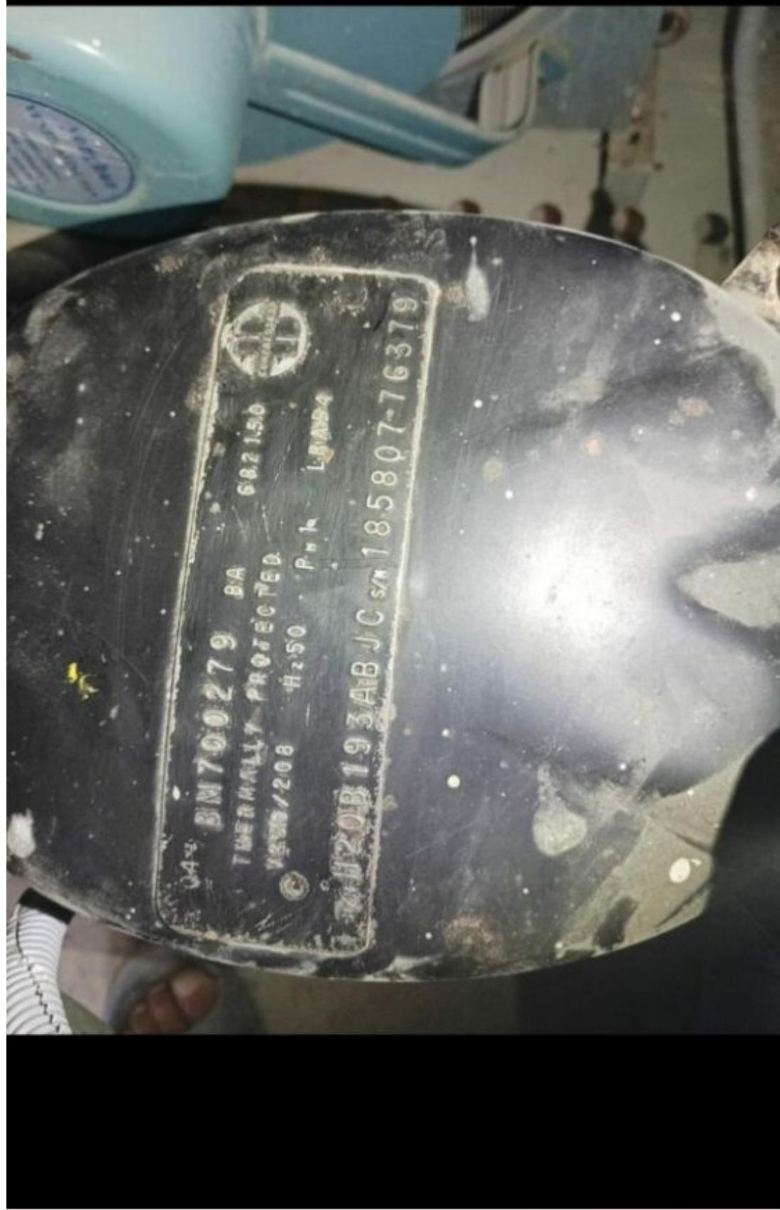
Mbsm.pro, Bristol, Compressor, H20B243ABC, 24000 btu, r22, 220 v 50hz, 2 ton , D6789205, AB5522G,
