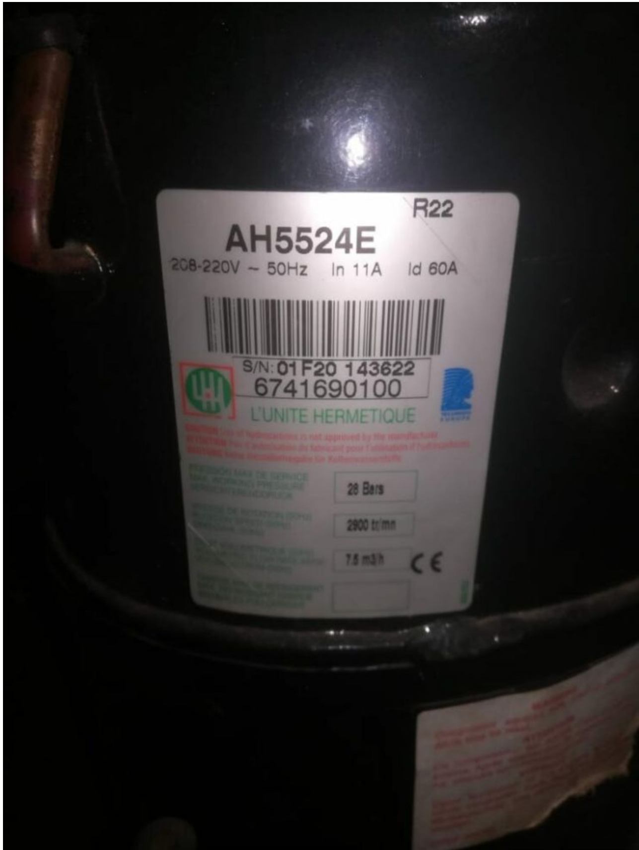
Mbsm.pro, Compressor, Tecumseh, AH141FT-014, R22, AH5524E, 2HP, 2Ton, 24200 Btu
