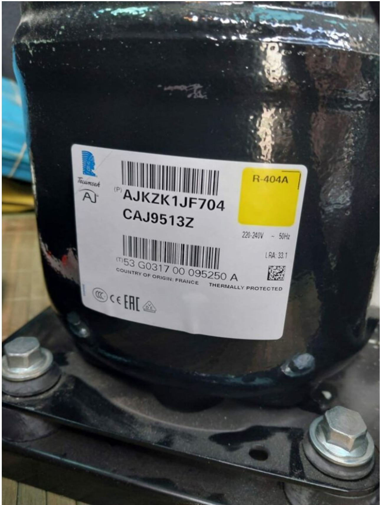
Mbsm.pro, Compressor, 1 1/8 HP, Hermetic, Piston, Tecumseh Compressor ,CAJ9513T, TAJ9513T, r404a / r22
