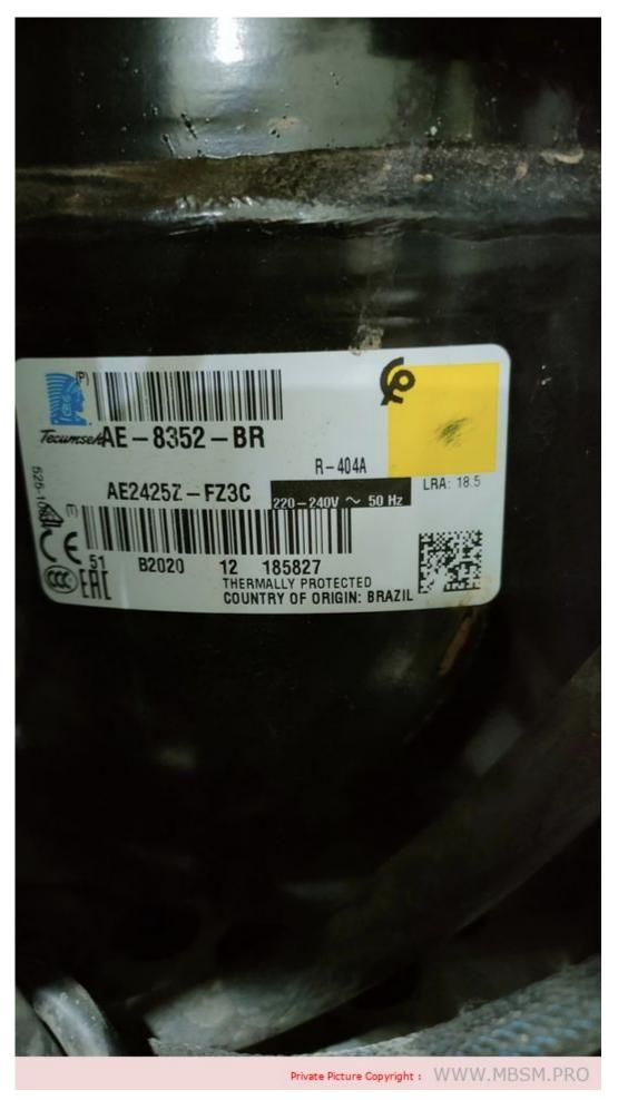
Mbsm.pro, AE2425Z-FZ3C , compressor, Tecumseh, R404A, 5/8 HP
