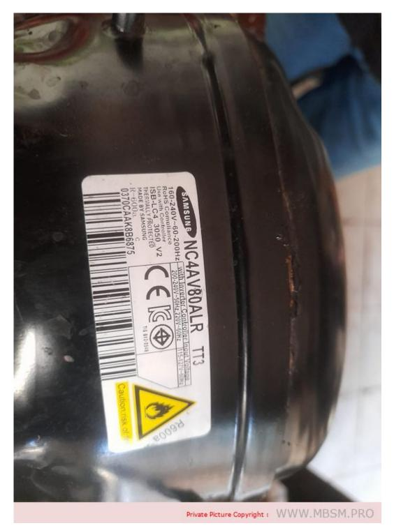
Mbsm.pro, Compressor, Samsung, Nc4av80alr, 1/4 hp, Displacement 8.08cc, Inverter, type Nc, R600a, Lbp, serie AV, Blcd Control 9 slot
