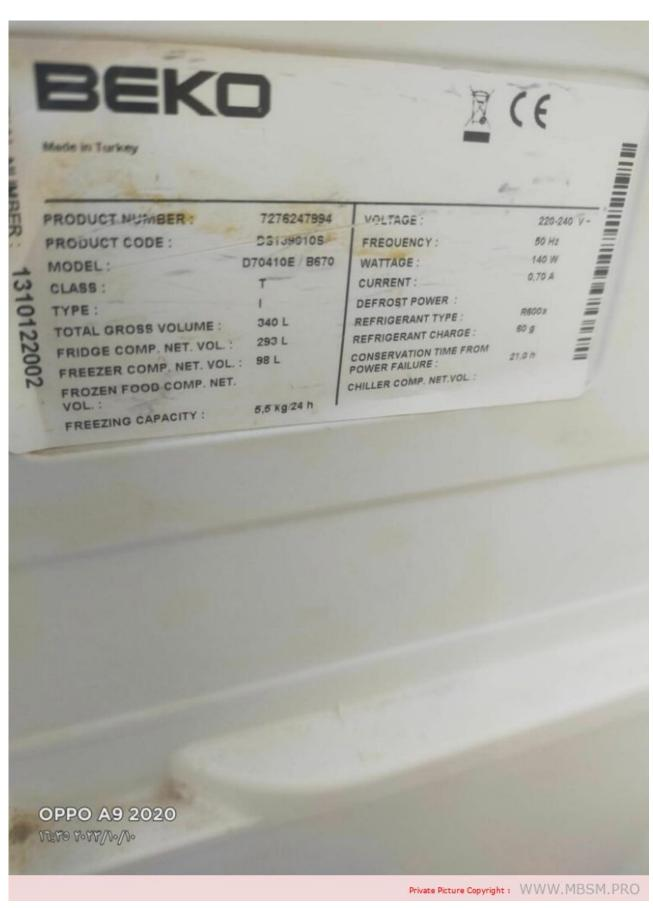
Beko, refrigerator, DS13901S, D70410e, b670,340 L, Compressor Acc, hmk95at, 1/5 hp, r600a, 80 g, 160 w
