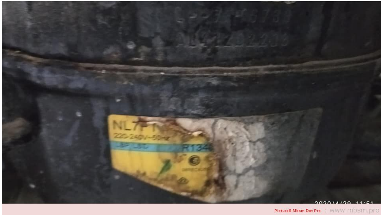
Danfoss ,Fridge Compressor ,NL7FT , 1/4 HP ,R134a
