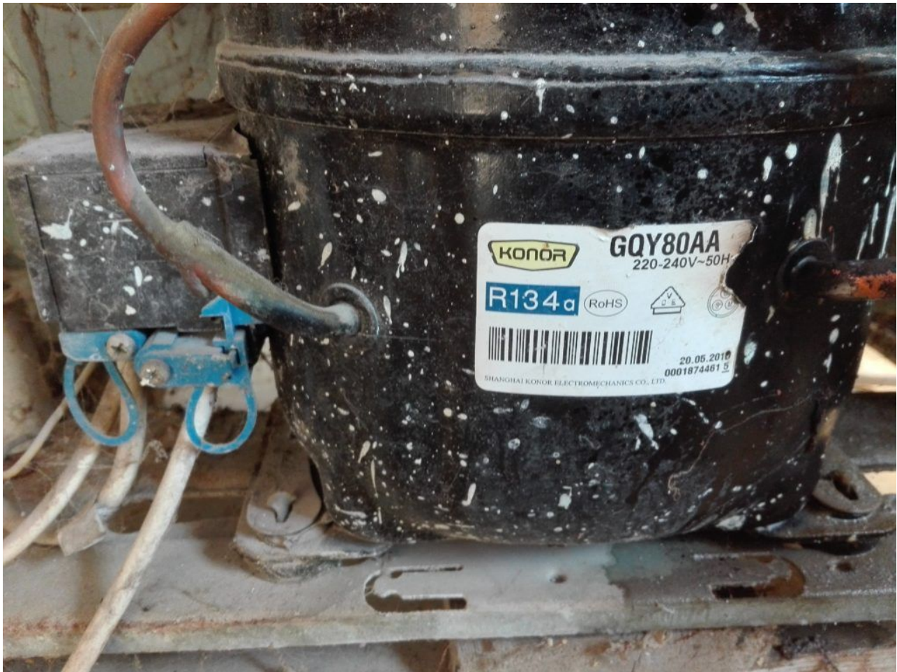
Compressor, KONOR, GQR90AA, R134a, 220-240V 50Hz, LBP , RSIR, 10,1kg 1/4HP, 220W
