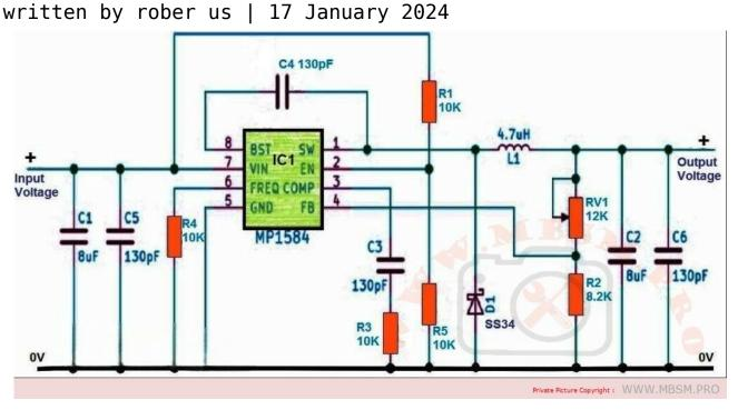
Mbsm.pro, 3A Adjustable voltage regulator circuit from 12 v to 5 v DC  $\,$
