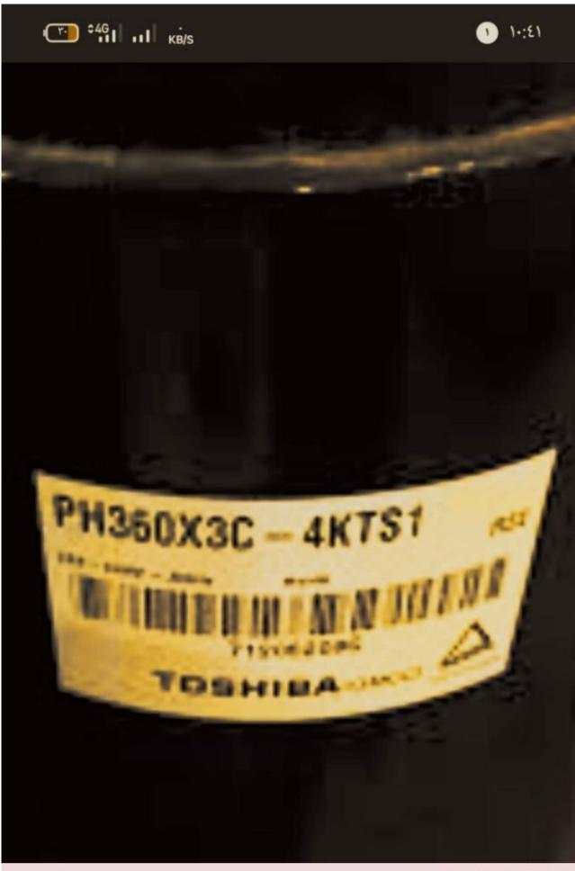
Mbsm.pro, Toshiba, Rotary, refrigerator ,compressor, PH360X3C-4KTS1, 1.5T++, 3 hp, 1 ph, r22
