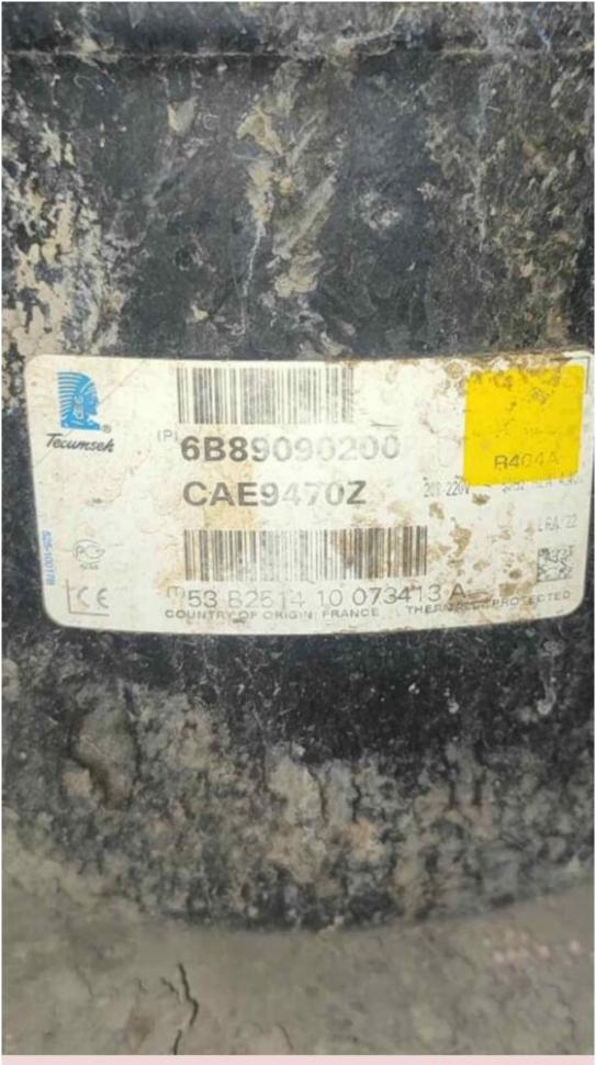
Mbsm.pro, Compressor, Tecumseh, 1/2 hp, CAE9470Z, (POE), HBP, R404A, 220-240V/1/50Hz , replaced by AE4470Z
