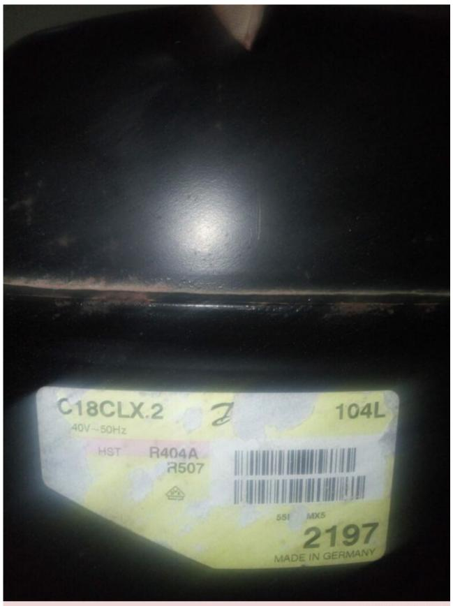
Mbsm.pro, compressor, Secop, SC18CLX.2, 104L2197, Danfoss R404A, R507, 3/4 hp, lbp
