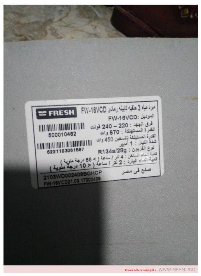
Mbsm.pro, FW-16vcd, FRESH WATER, DISPENSER, 3 SPIGOTS, COLD/HOT/WARM, Compressor, 1/10 hp, r134a, 28 g
