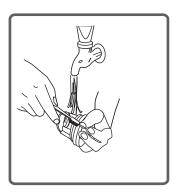
• After cleaning the filter, fit the filter cover and tighten it by rotating it in clockwise direction.
