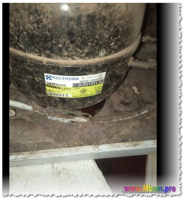
c-bzN101 appears to be a model number for a KULTHORN refrigerator compressor. It's specifically a 1/8HP compressor, which is commonly used in smaller refrigerators.
