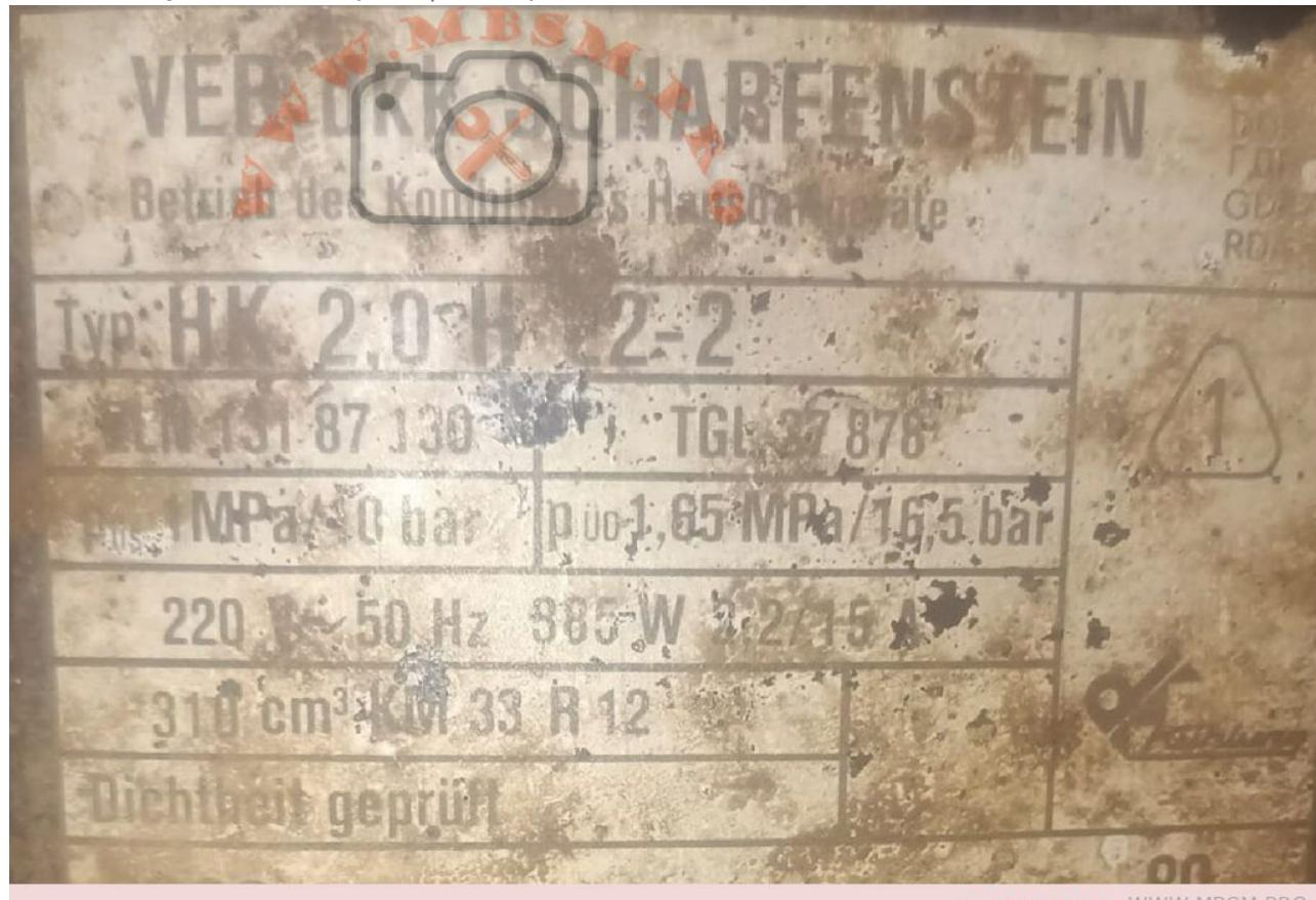
Mbsm.pro, Compressor, tgl27878, tgl27 878, VEB dkk Scharfenstein, 1993, R12, 3/8 hp++, 1/2 hp-, 385 w, Cooling Compressor, 0 °C 10 °C, Replaced by GP12TB
