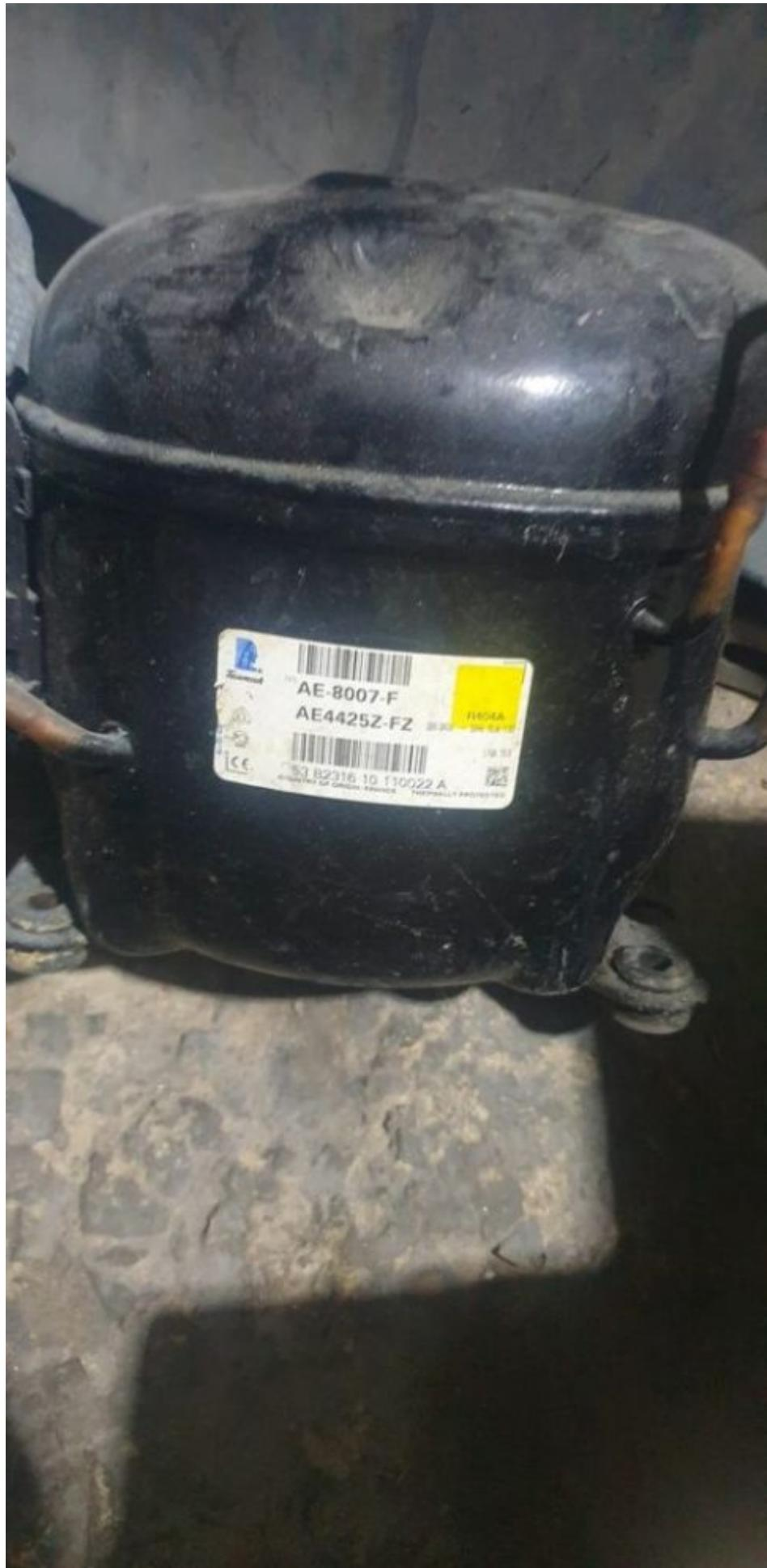
Mbsm.pro, Compressor Tecumseh, AE 4425 Z , AE-8007-f, AE4425Z-FZ, H/MBP, AE 4425 Z, AEZ 4425 Z, 1/5 hp++, 1/4 hp-, r404a
