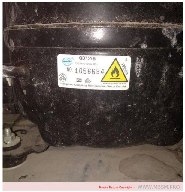
Mbsm.pro, Refrigerator, Electrolux, 308 Liters, Silver, Ert45g2hqi, Compressor, QD Compressor, R600a, QD75Y, 1/6HP,
