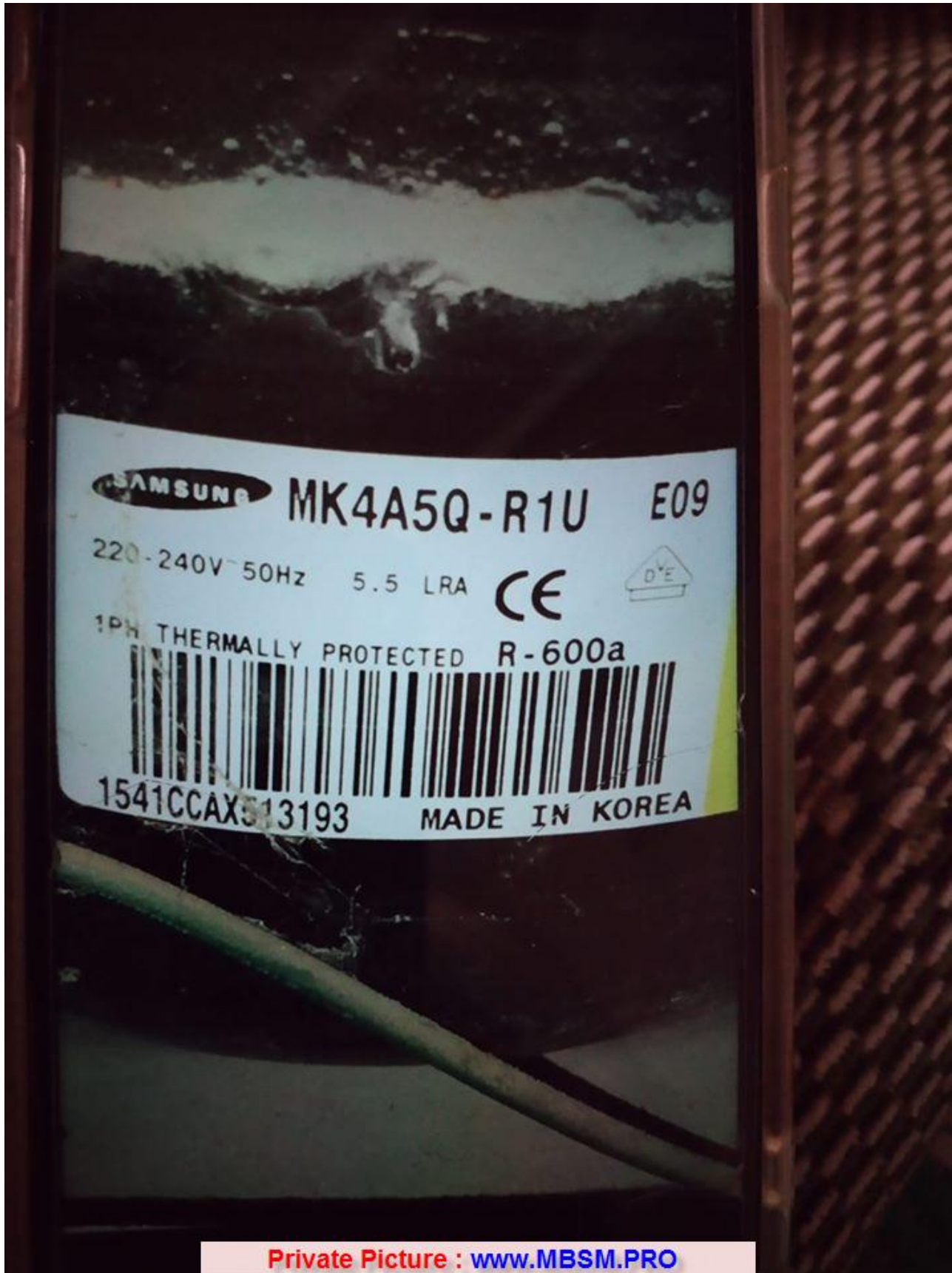
Compresseur, Samsung , 1/5 HP, 155/160w , r600a ,220/240v~50, Mk4a5qr1u, Mk4a5q-R1u, 5.5Lra, 1PHASE
