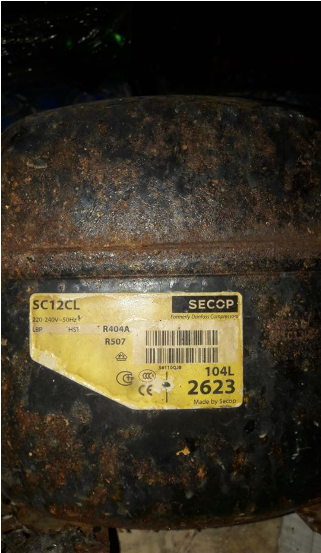
Compressor Danfoss SC12CL 3/8 HP , LBP/MBP, R404A/R507
