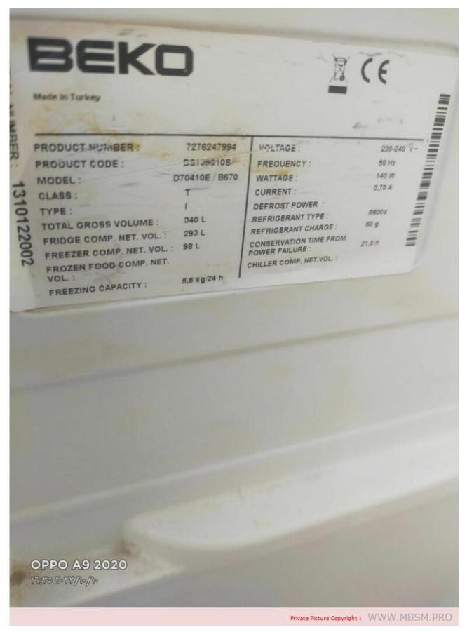
Beko, refrigerator, DS13901S, D70410e, b670,340 L, Compressor Acc, hmk95at, 1/5 hp, r600a, 80 g, 160 w
