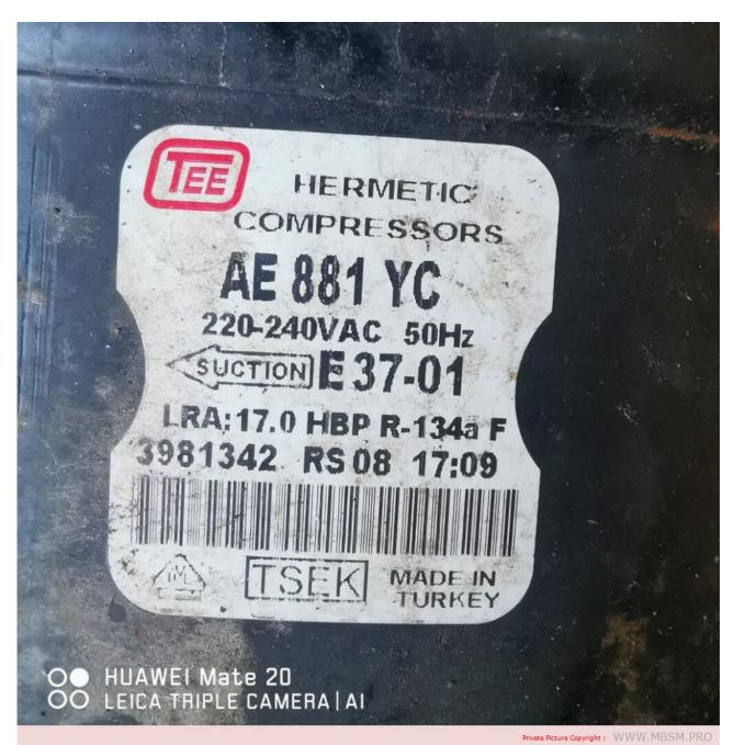
Mbsm.pro, Tee compressor , AE881YC, AE 881 YC, 881 kcal, 1024 w, Hbp, 1/3 hp++, 220-240VAC 50Hz, LRA: 17.0, MADE IN TURKEY
