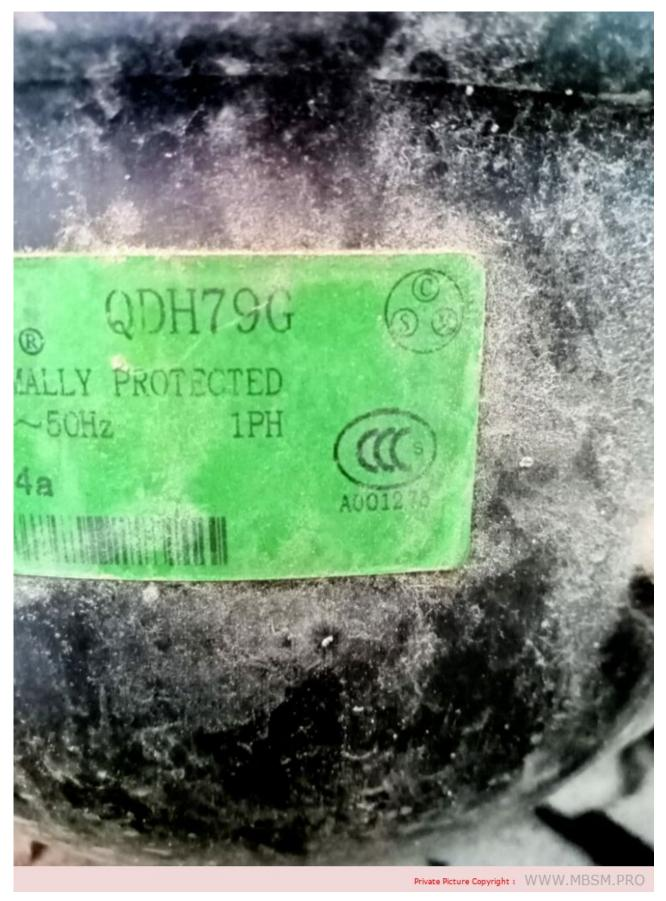
Mbsm.pro, Compressor, Qdh79g, 1/4 Hp, 205 w, Lbp, R134a, 220v, 1 phase 50 hz, QDH79G Refrigerator
