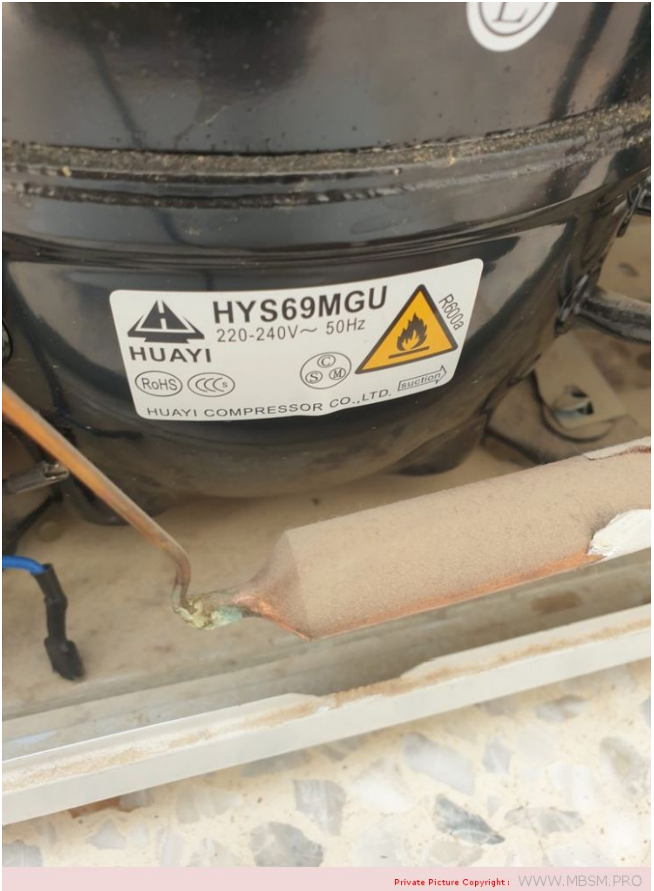
Mbsm.pro, Compressor, HYS69MGU, 1/6 hp, R600, 120 W, R600a-LBP 220-240V~50Hz
