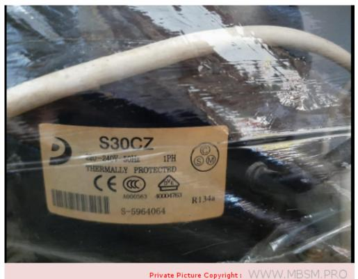
Mbsm.pro, Compressor, DONPER, Refrigeration, S30CZ, R134a, 1/12 HP, LBP, 220V-240V 50HZ, Disp. 3.0cc
