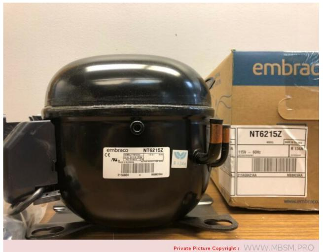
Mbsm.pro, Compressor, Embraco, Refrigeration, NT6215Z, 1/2 Hp, MHBP, Big ++, R134A, CSIR, 115 V
