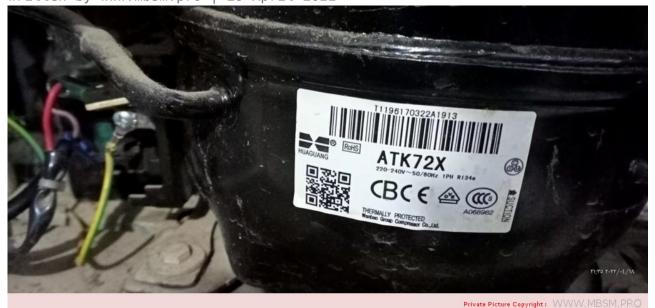
Mbsm.pro, Compressor, atk72x, HuaGuang, cmA069LHEM, LG, lbp, 1/4 hp, 205 W, 699 Btu/h, 220-240V 50HZ, Refrigerator, Fresh, FNT-BR470K, 1 A, 376 L, R134a, 95 G, freezer
