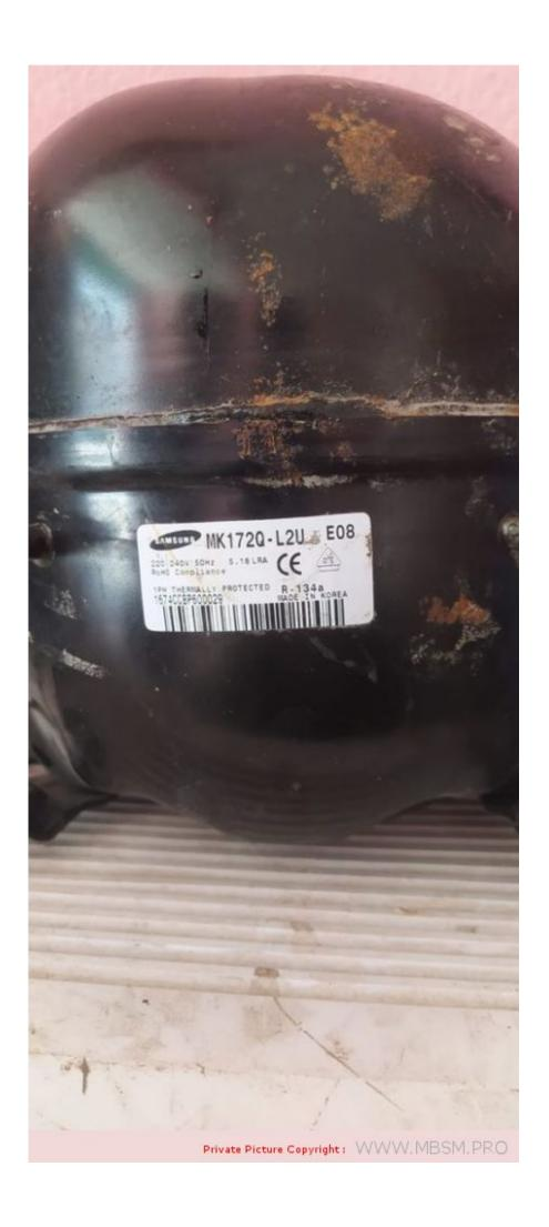
Mbsm.pro, Compressor, Mk172Q-L2U, 1/4 Hp, 205 W, 699 BTu/H, Samsung Compressor, Mk Serie, R134A, 7.21 cc, 220-240 v, LBP, Static Compressor, RSIR
