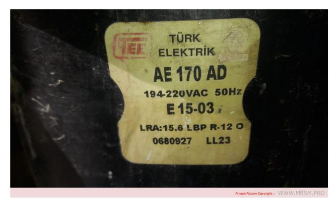
Mbsm.pro, Compressor, Tee compressor, ae170ad, ae170ac, ae170ap, 150 w, 1/5 hp, r12
