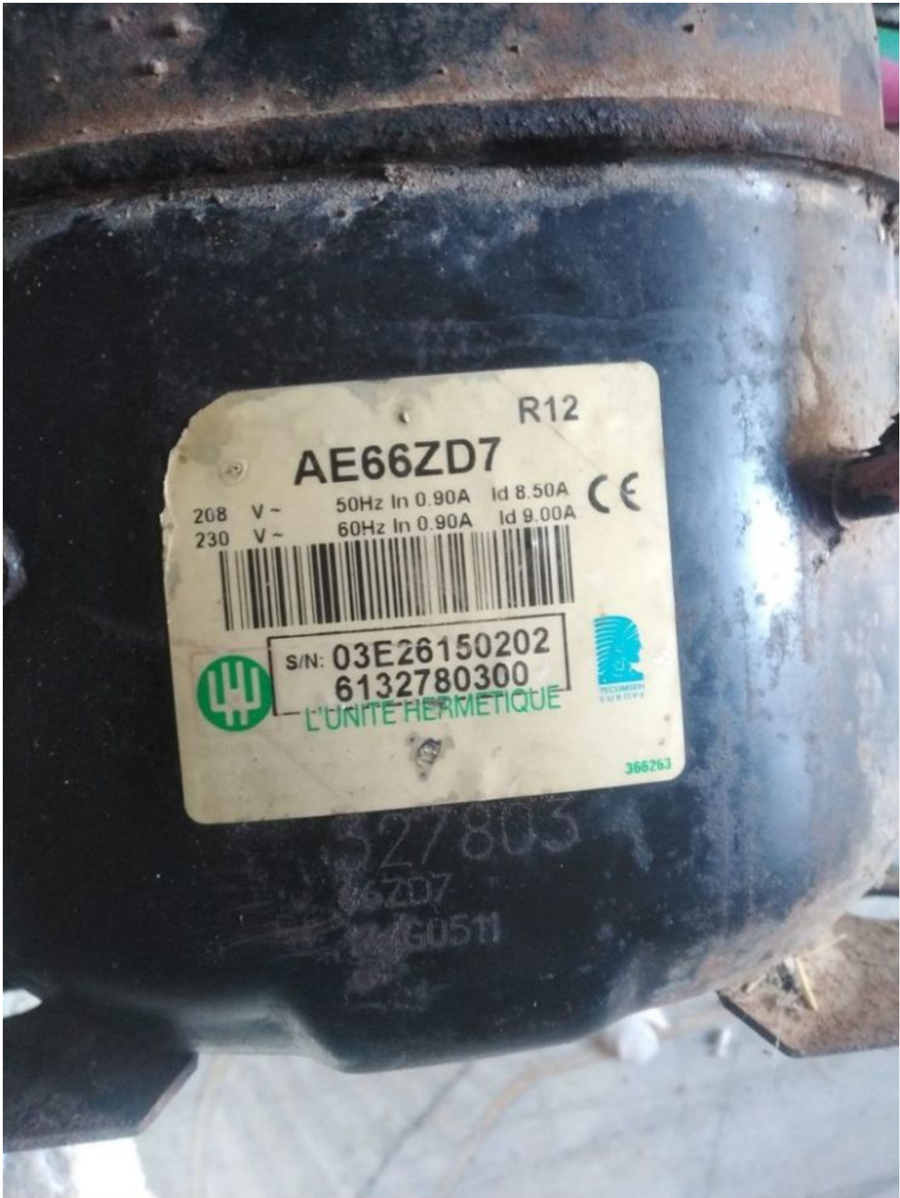
Mbsm.pro, Compressor, AE66ZD7, Tecumseh 1/6 HP, 115V, 450 BTU, R12, Hermetic
