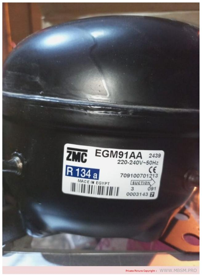
The EGM91AA is a hermetic reciprocating compressor manufactured by ZMC, designed primarily for use with R134a refrigerant. It operates on a voltage range of 220-240V at 50Hz and is typically used for low back pressure (LBP) refrigeration applications like household refrigerators and freezers.  $\Box$
