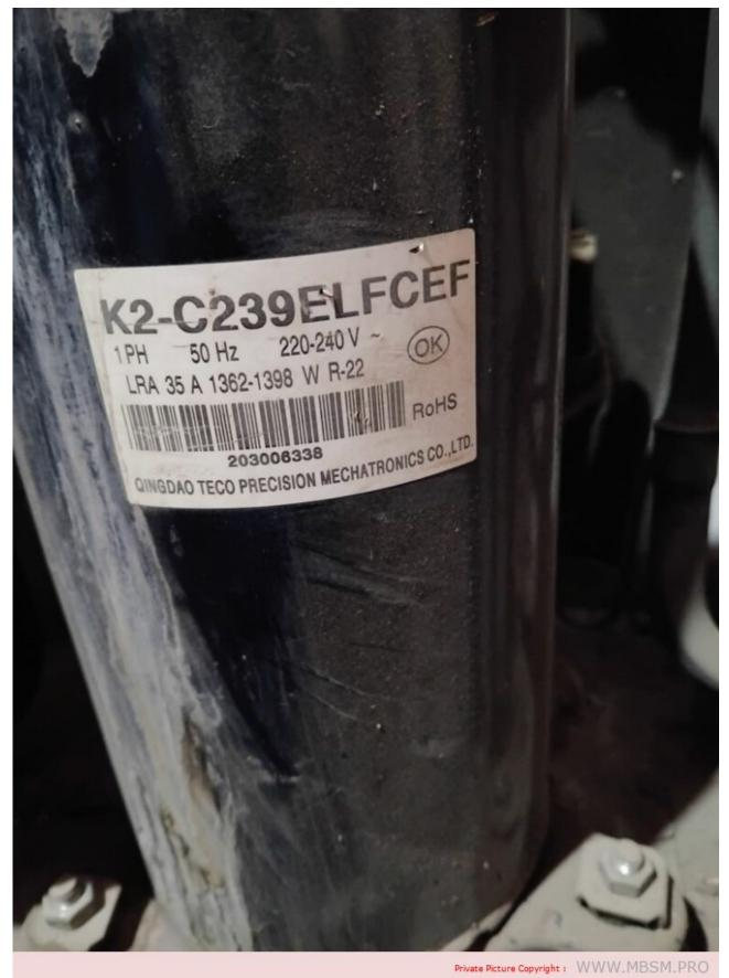
The **K2-C239ELFCEF** appears to be a model of an air conditioning or refrigeration compressor. Based on the search results, here is the relevant information:
