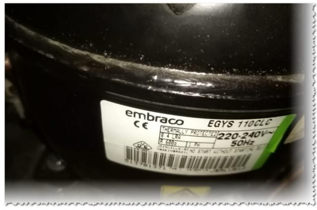
The **EGYS110CLC** compressor has a power rating of 1/3 HP (horsepower) and is designed for low-temperature applications. Here are some key specifications related to its horsepower and performance:
