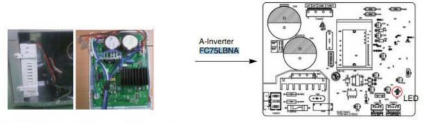
\* There is a PCB located in the PCB case next to the compressor. That is the driver PCB. the linear compressor.
