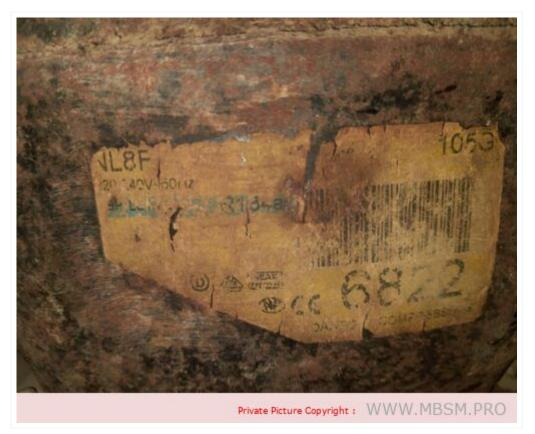
The search results provide information on two different topics: a compressor with model number 105G6822 and an adhesive product called ET-HP. The compressor is a Secop NL8F model with a power of 1/4+ Hp and a displacement of 8 cc, using R134a LBP gas. ET-HP Adhesive is a two-part epoxy used to anchor threaded rod and rebar in concrete applications.
